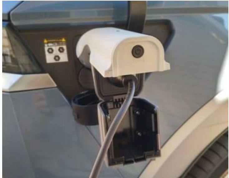
Figure 2:6: V2L using an adapter for Hyundai Ioniq 5 6
