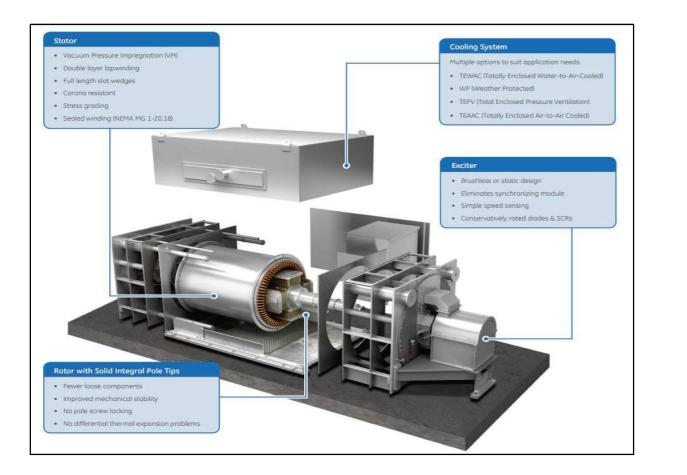
Figure A2.1 Assembly diagram showing synchronous condenser
