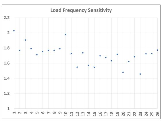
Figure 9.11 Load frequency sensitivity assumed for the 26 events to arrive at the validation plots
