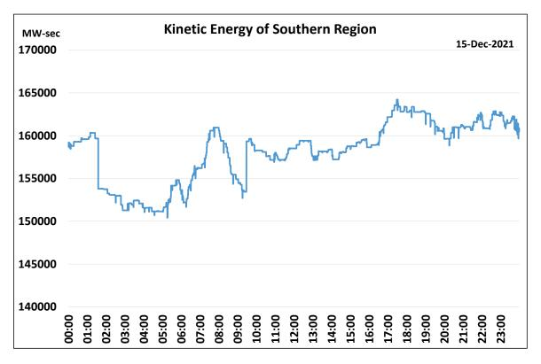
Figure 7.11 Sample daily kinetic energy curve for SR
