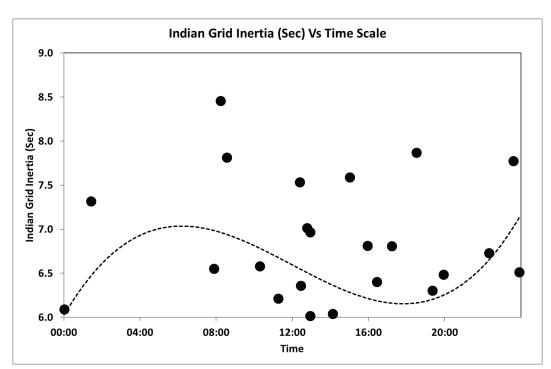
Figure 6.3 Grid Inertia vs Time of Day
