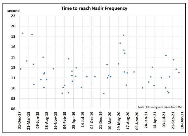
Figure 8.4 Observed time to reach nadir frequency during events
