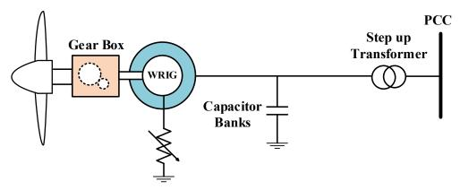
*Figure 4.9 Variable-speed, wound rotor induction generator (Type-2 WTG)*
