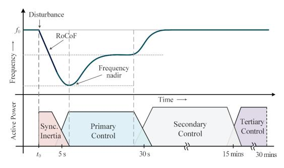
Figure 1.1 Stages of power system frequency response after a disturbance
