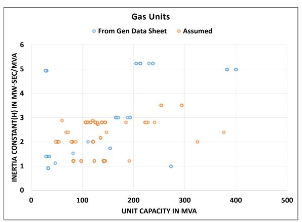
Figure 4.4 Inertia constant of Gas Generators in India
