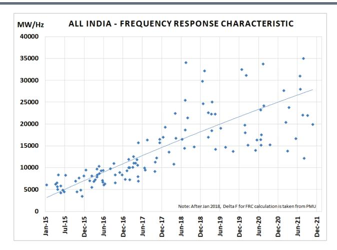
Figure 8.6 Frequency Response characteristics observed during grid events in India
