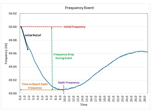
Figure 5.4 Approximate frequency response and other parameters of centre of inertia
