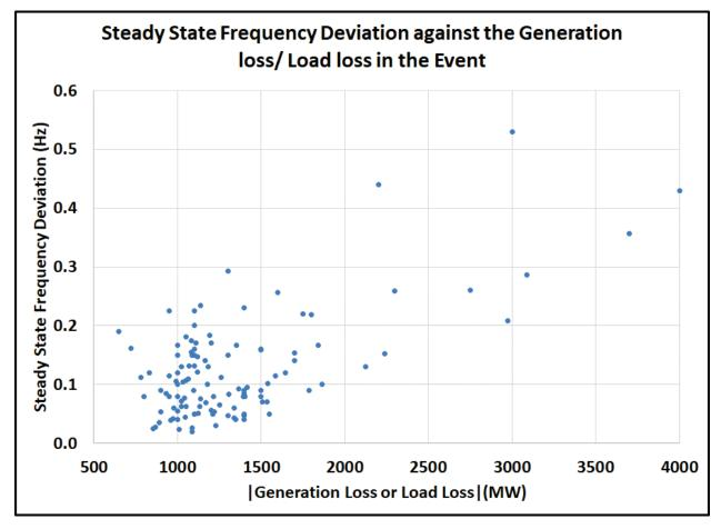
rate at which the primary response is activated after a disturbance. The parameter has been plotted against the generation loss/load loss during the events as given in Figure 8.5.
