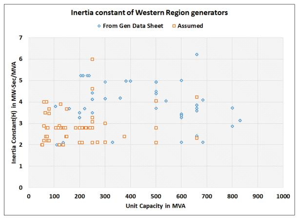
Figure A1.2 Inertia Constant of Western Region Generators
