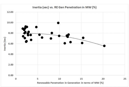
Figure 6.4 RE Penetration Vs Grid Inertia
