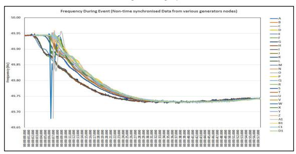
Figure 5.5 Typical time synchronization issues in high resolution frequency data
