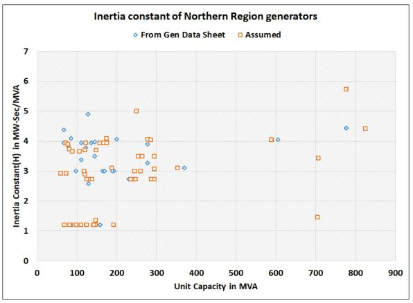
Figure A1.1 Inertia Constant of Northern Region Generators
