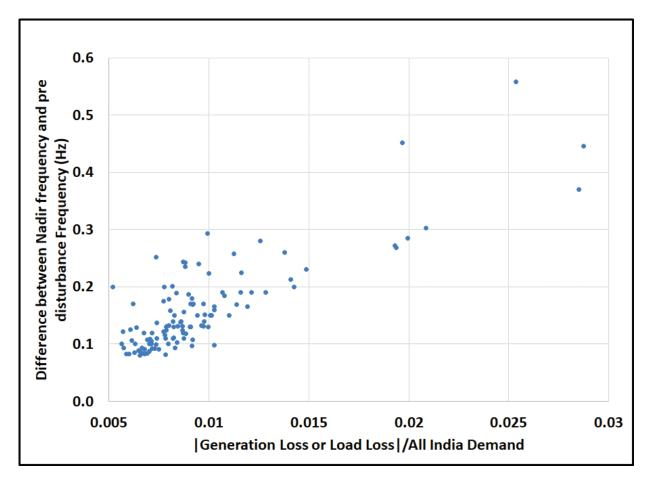
Figure 8.3 Maximum frequency deviation vs. normalized power imbalance
