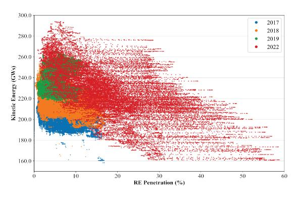
Figure 9.1 Variation of WR kinetic energy wrt RE Penetration
