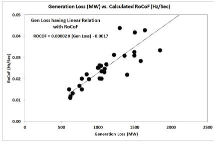
Figure 6.5 Generation Loss vs. Frequency Drop
