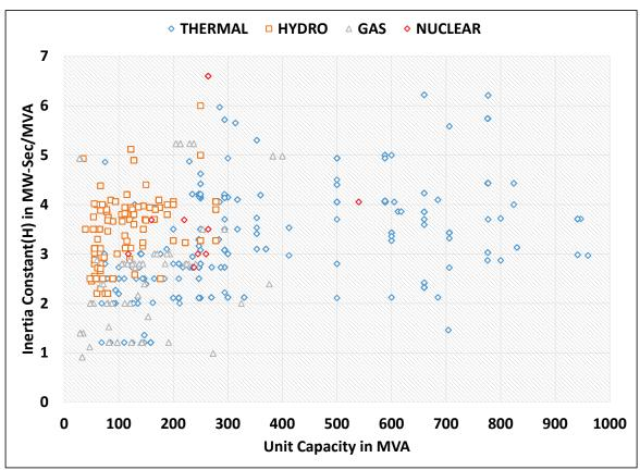
Figure 4.6 Inertia constant of generators in India
