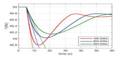
Figure 2.4 Impact of diminishing inertia on system frequency response [2]
