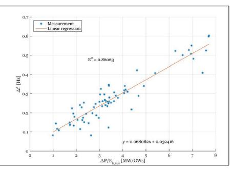
Figure 3.2 Maximum frequency deviation relative to power imbalance and estimated kinetic energy
