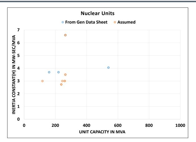
Figure 4.5 Inertia constant of Nuclear Generators in India
