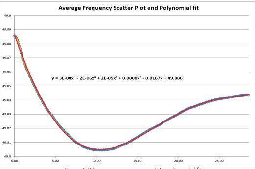
Figure 5.3 Frequency response and its polynomial fit
