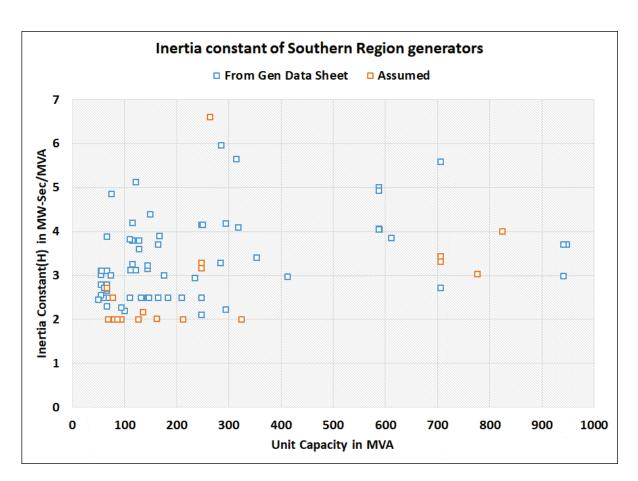
Figure A1.3 Inertia Constant of Southern Region Generators
