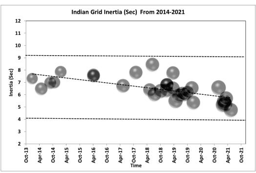
Figure 6.2 Grid Inertia on Year Scale
