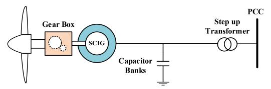
Figure 4.8 Fixed-speed, squirrel cage induction generator (Type-1 WTG)
