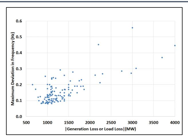
Figure 8.2 Maximum frequency deviation vs. power imbalance
