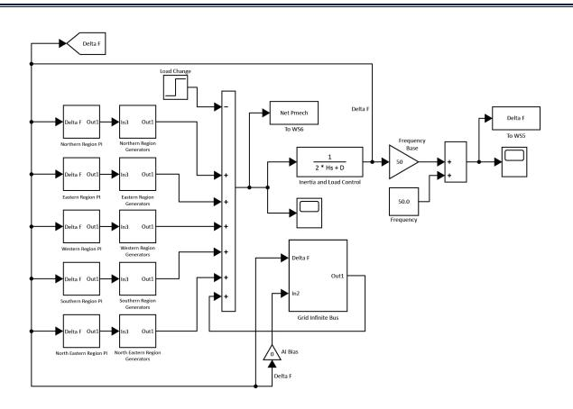
Figure 9.8 Multi-Region integrated Frequency Control model
