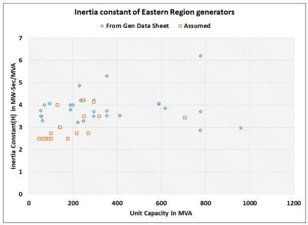
Figure A1.4 Inertia Constant of Eastern Region Generators
