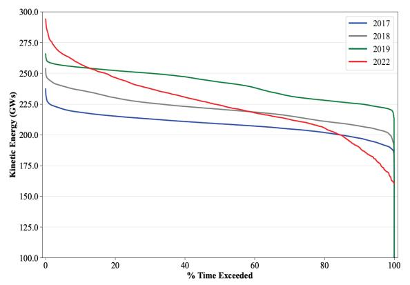
Figure 9.3 Duration Curve of Kinetic Energy
