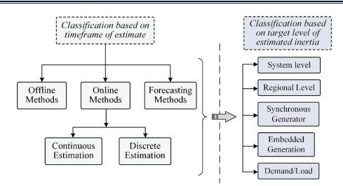
Figure 2.6 Classification of inertia estimation methods
