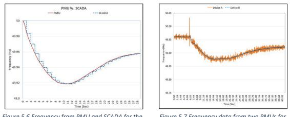
Figure 5.6 Frequency from PMU and SCADA for the same event
