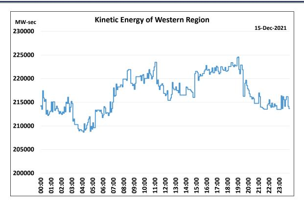
Figure 7.10 Sample daily kinetic energy curve for WR
