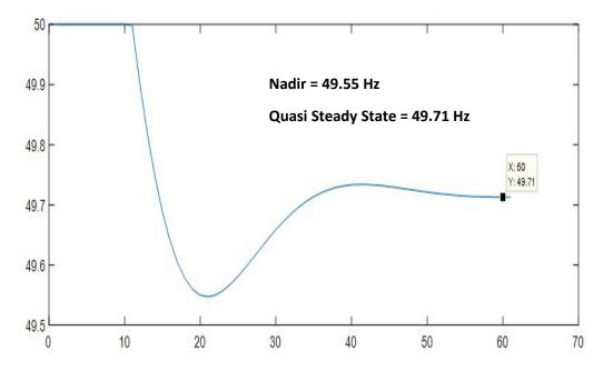
Figure 9.12 System frequency after reference contingency event of 4500 MW perturbation
