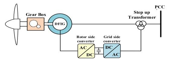
Figure 4.10 Variable-speed, doubly fed induction generator (Type-3 WTG)
