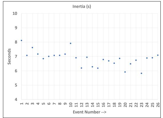
Figure 9.10 Inertia assumed for the 26 events to arrive at the validation plots
