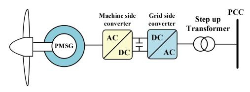
Figure 4.11 Variable-speed, permanent magnet synchronous generator (Type-4 WTG)
