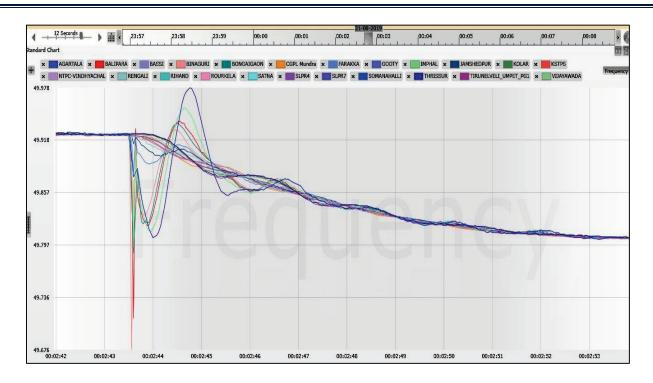
Figure 8.1 Frequency behaviour at different locations across the grid for generation loss event
