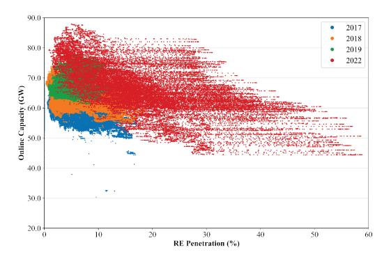
Figure 9.4 Online synchronous capacity of Western Region wrt RE penetration
