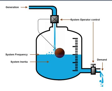
Figure 2.1 Power system inertia and water tank analogy
