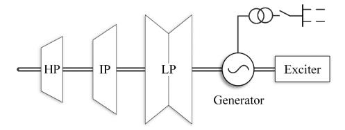
Figure 2.3 Drive train of a thermal power plant with three pressure stages.
