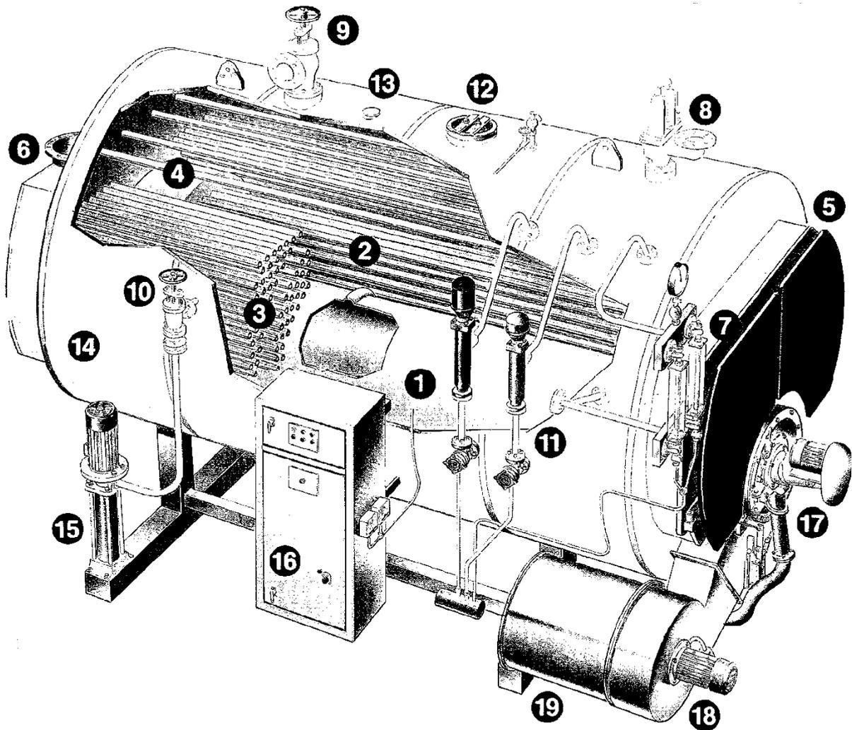
**Fig. 1 A typical smoke tube package boiler**
