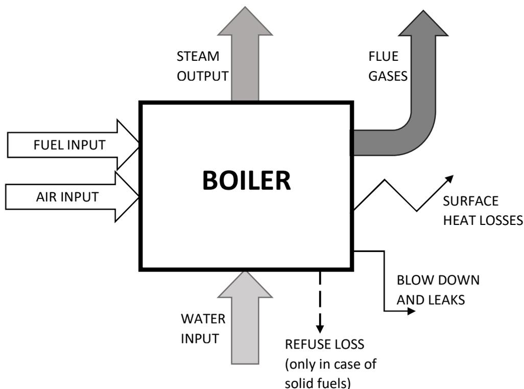
**Fig. 3** Input and output streams and the heat losses of a boiler
