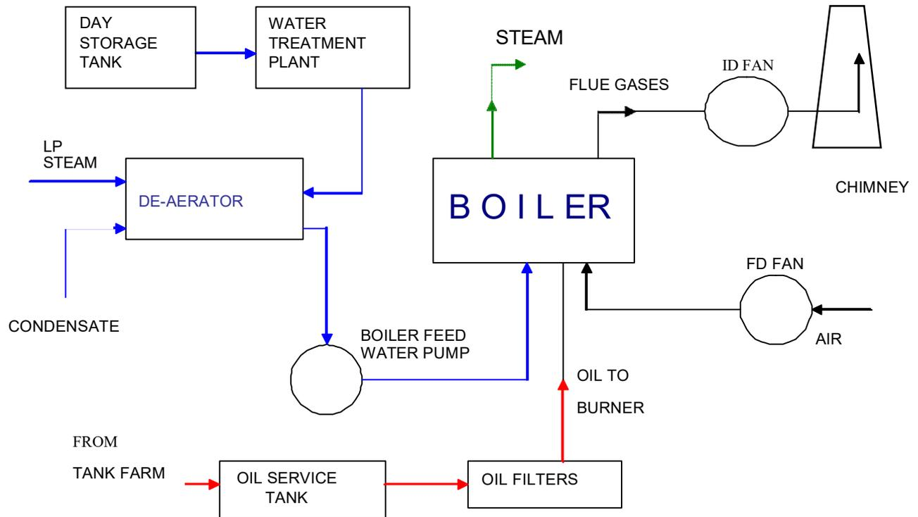
**Fig. 2 Components in a boiler system**
