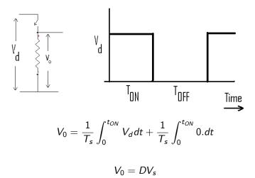
D is defined as the ratio of on time to total time and is given by  $D = \frac{T_{on}}{T_{sol}}$
