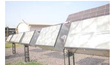
High Efficiency & high concentration small area solar cell modules on 2D Tracker installed at SERE
