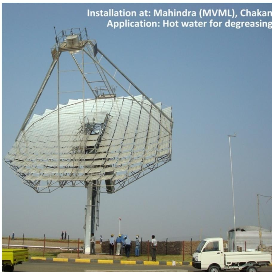
ARUN 160 at automobile plant of Mahendra, Chakan, near Pune with pressurized hot water for degreasing
