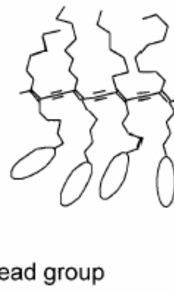
Figure 7. Illustration of the "side chain disorder" model to explain the chromatic property of polydiacetylenes.
