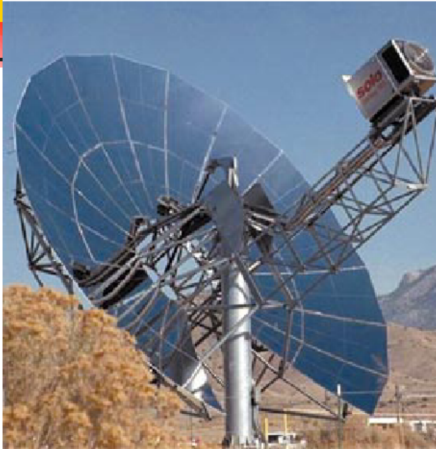
The Advanced Dish Development System is a 10 kW water pumping system developed by WG Associates for use by Native Americans in the southwest U. S.
